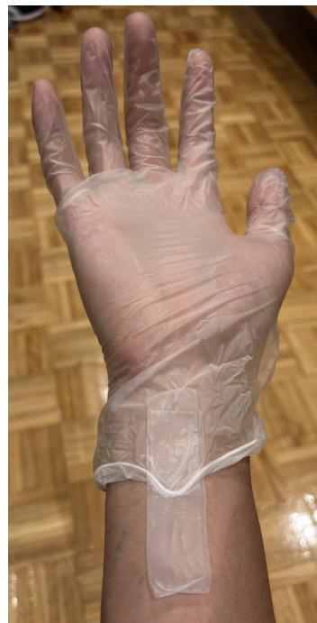
Figure 19: The first tape doffing design
