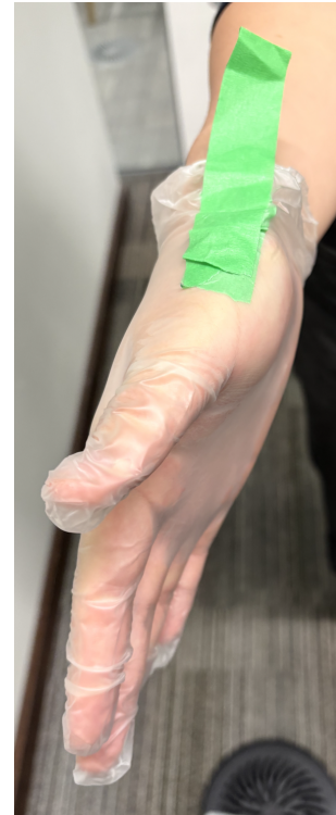
Figure 21: The Final tape doffing design
