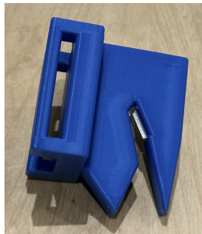
Figure 5: 4th iteration of glove slicing design
