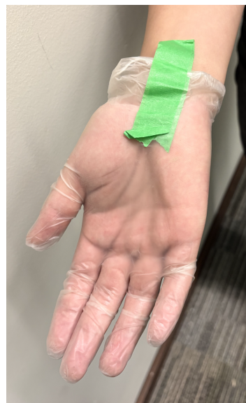
Figure 20: The Second tape doffing design
