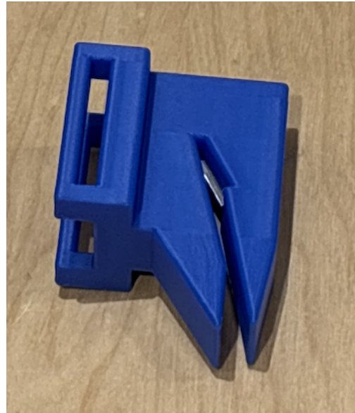
Figure 14: 3rd iteration of glove slicing design
